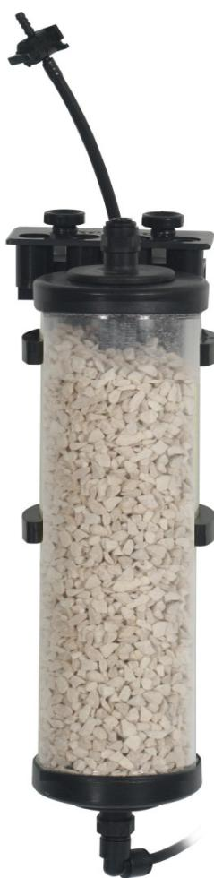
The **Hydrocarbonatreactor** is a ready to use filtration system that is post-switched to a sulphur reactor to neutralize the sulphuric acid, produced by the sulphur reactor.
